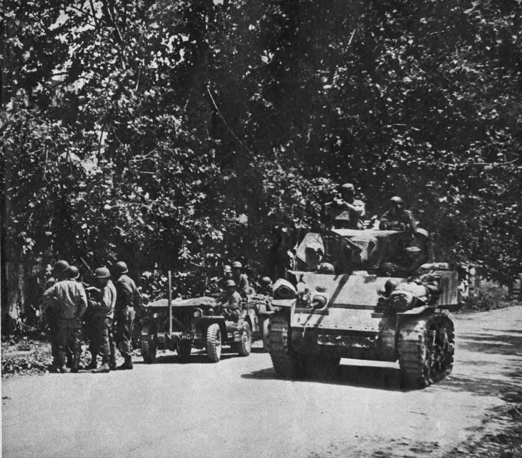
The M-5A1 is the standard American light tank. The tank's suspension, like that of the M-8 gun motor carriage shown at the left, consists of two pairs of tandem bogie wheels, a large trailing idler set flat on
